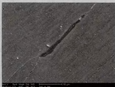
(a) 裂纹形貌
